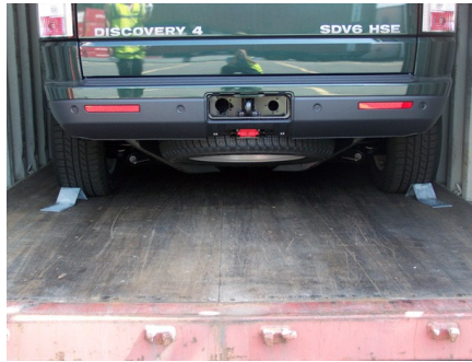
...secure metal chock to container floor.
