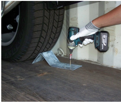
Using metal chocks, screws and power screwdriver...
