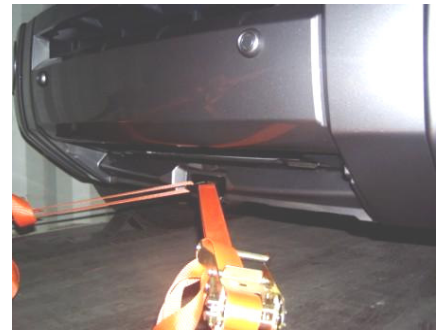
Once chocked ensure vehicle is correctly lashed
