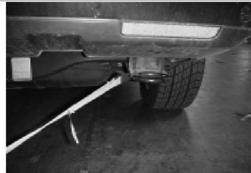
Rear right lashing point
