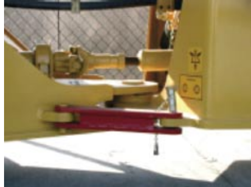
Safety lock for: articulated haulers motor graders wheel loaders
